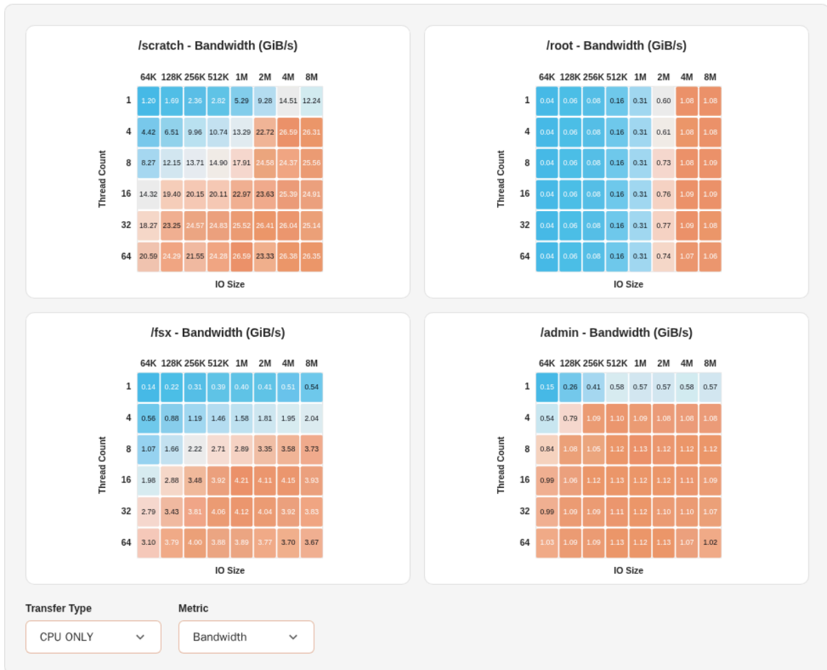
Figure 17 · Interactive heatmaps comparing storage system performance (scratch, root, FSx, admin) across different thread counts and I/O sizes. Visualizes throughput (GiB/s) and IOPS to identify optimal configurations for each storage tier.
